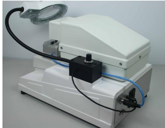
Opti-Cal cable routing
